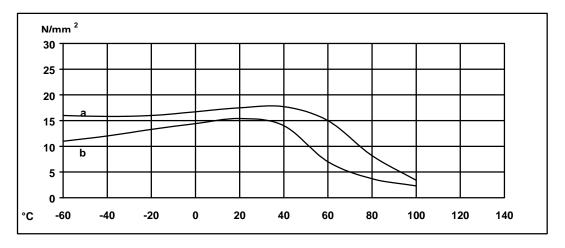
Roller peel test (ISO 4578)
